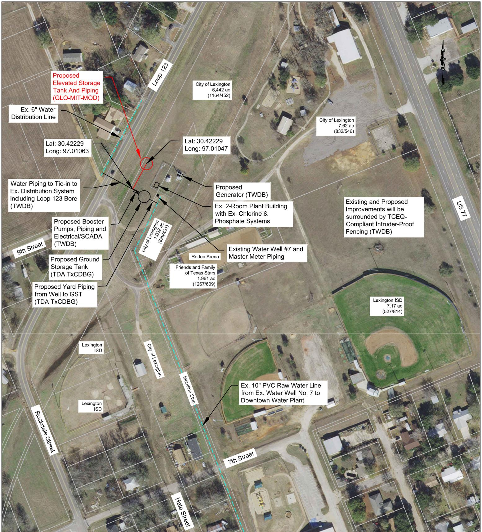
Proposed City of Lexington Elevated Storage Tank is not drawn to scale and locations of improvements within the plant site may change once site field survey is performed. Even though they may change location, all improvements will be constructed on existing City-owned land. This Site Plan is for GLO Application & Environmental Purposes and not for Design.
